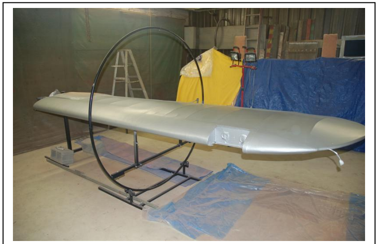
The Club's rotation fixture. Since Tripacers don't have wingtip attach points, the rotation ring attaches to the strut support fittings. If you're a member, you can use the fixture for four months. Cost? Shipping to the next user.
